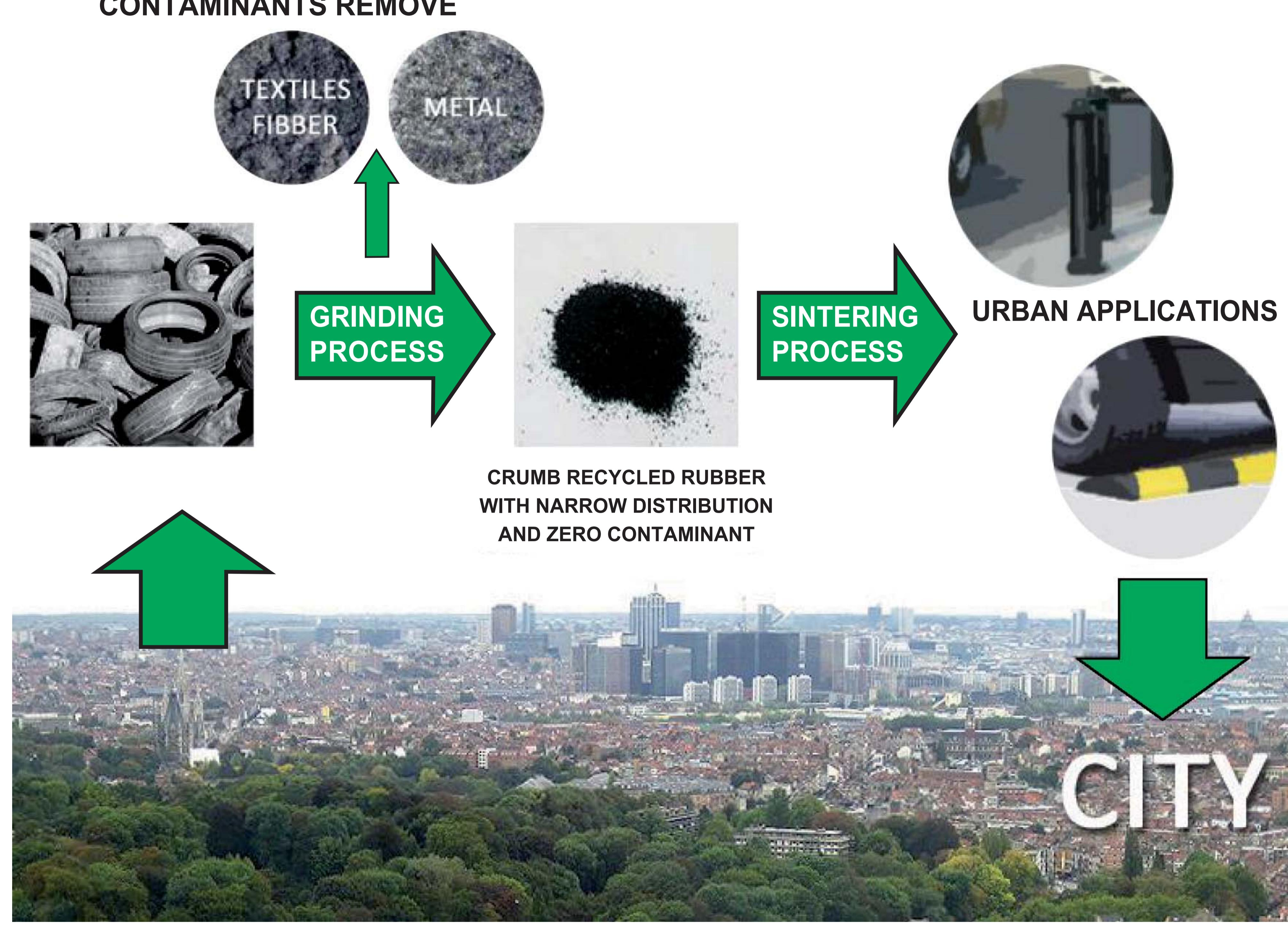
**The main goal is to adapt the current industrial rubber recycling process to supply innovative recycled rubber urban furniture products manufactured by an innovative sintering process as an alternative to virgin rubber, wood or concrete products.**
